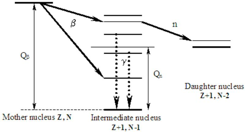
Fig. 3. The diagram of decay of an atom emitting the delayed neutron.
